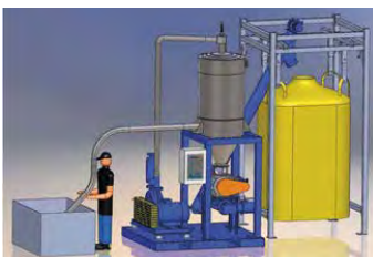
Silo loading units working with the Suction Pressure Principle
