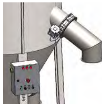
Pneumatic Discharge Valve + Control
