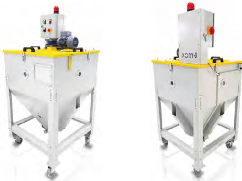
Mixer with touch screen control
